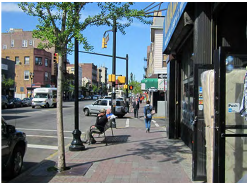
Bergenline Avenue Sidewalks have a Furnishing Zone that is utilized as shown in this photo, but the Pedestrian Zone and Frontage Zone are of Limited Width
